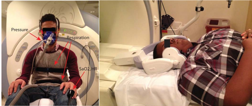
FIGURE 1: Experimental setup for airway collapsibility measurement. Left: A facemask covering nose and mouth is connected to an external hose, which contains an inflatable balloon. Once expanded, the balloon can block the air flow and serve as external inspiratory load. Physiological signals including facemask pressure, chest and abdomen displacements, oxygen saturation, and heart rate are simultaneously recorded and synchronized with MRI acquisition. Right: Positioning of the six-channel receiver coil. Note that subjects in this study wore all equipment shown in both panels.
