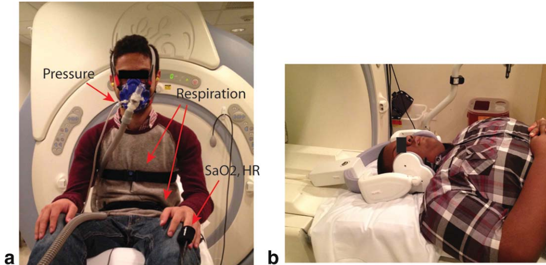
FIG. 1. Experimental setup for the proposed sleep MRI. a : Placement of the devices on a subject. The tube-mask setup necessary for the airway occlusion test is shown. Pressure from the mask port is transmitted via the thin transparent tube to a metallic pressure transducer which is approximately 8 m away from the scanner. Respiratory belts are placed around the subject's chest and abdomen. Oxygen saturation and heart rate are monitored using the MR compatible optical finger plethysmograph. b : The six-channel carotid coil on a pediatric subject. In our experiments, the left and right side of the coil are each wrapped with a pillowcase to avoid a contact between the coil and subject's face.
