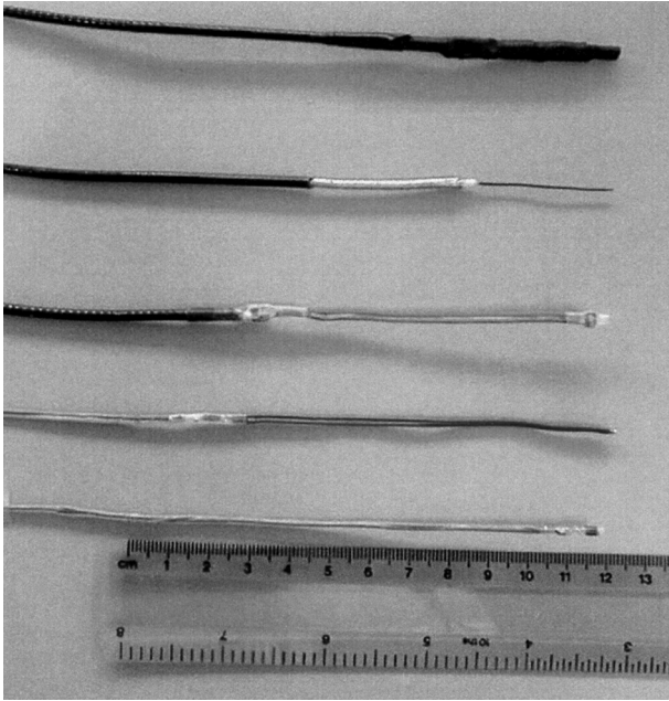
Figure 2. Catheter coils. From top to bottom: opposed solenoids, loopless probe, twin lead, coax-stub-matched twin lead, and coax-stub-matched single solenoid.
