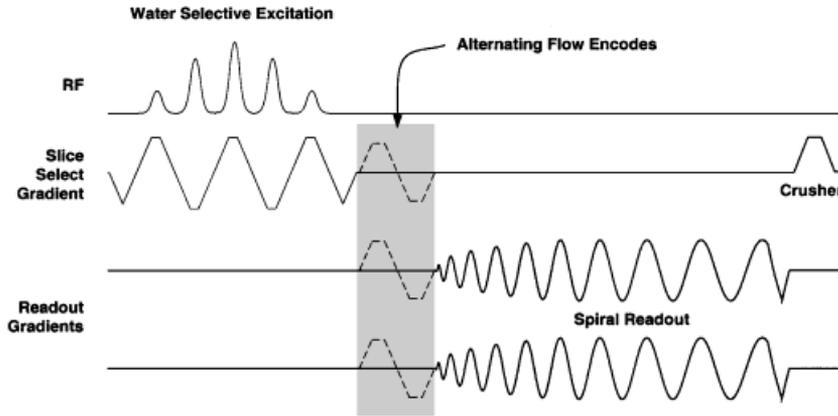
FIG. 1. Real-time color flow pulse sequence. A low flip-angle excitation (water selective spectral-spatial excitation is shown) is followed by velocity-encoding bipolars in  $x$ ,  $y$ , and  $z$ , which provide flow encoding along a prescribed direction. Finally, spiral-interleave readouts are used to cover  $k$ -space, and a crusher dephases any remaining signal.
