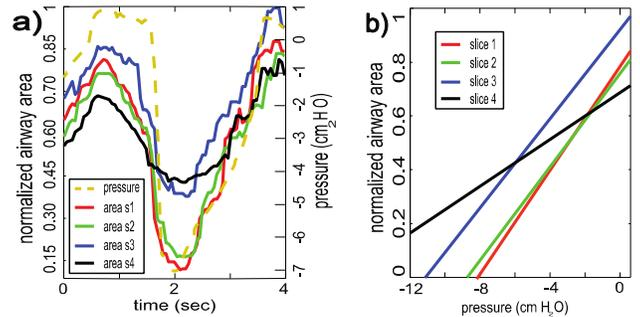
**Fig 2.** a) Plot of airway pressure and segmented airway areas at different locations. S1-S4 correspond to the slice from left to right in Fig. 1. b) Linear regression plots for all 4 slices. The slope is defined as compliance. Also note the projected closing pressure (airway area = 0).
