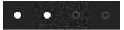
Fig. 1: From left to right: simulated lumen, lumen with noise \mathbf{s} + \mathbf{n} , and MF \hat{\mathbf{s}} . Lumen SNR = 75, W = 3.1 mm, 7% dilation, and \delta = 0.7 mm. High SNR is used to make \mathbf{s} apparent in noise.
