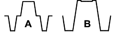
Figure 1: The two different readout waveforms used in the interleaved SSFP phantom experiments.
