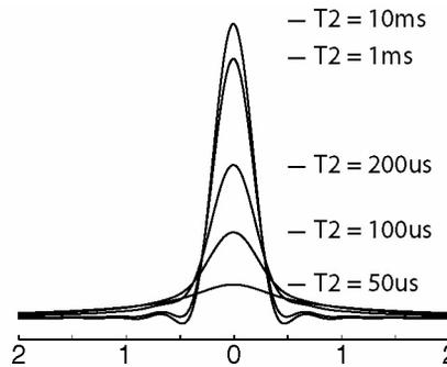
Figure 2: Simulated slice profile for 400 $\mu$ s-duration half-pulse.
