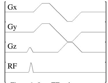
Figure 1: 8- $\mu$ s TE pulse sequence
